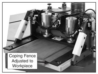
Figure 10. Workpiece positioned on jig.
